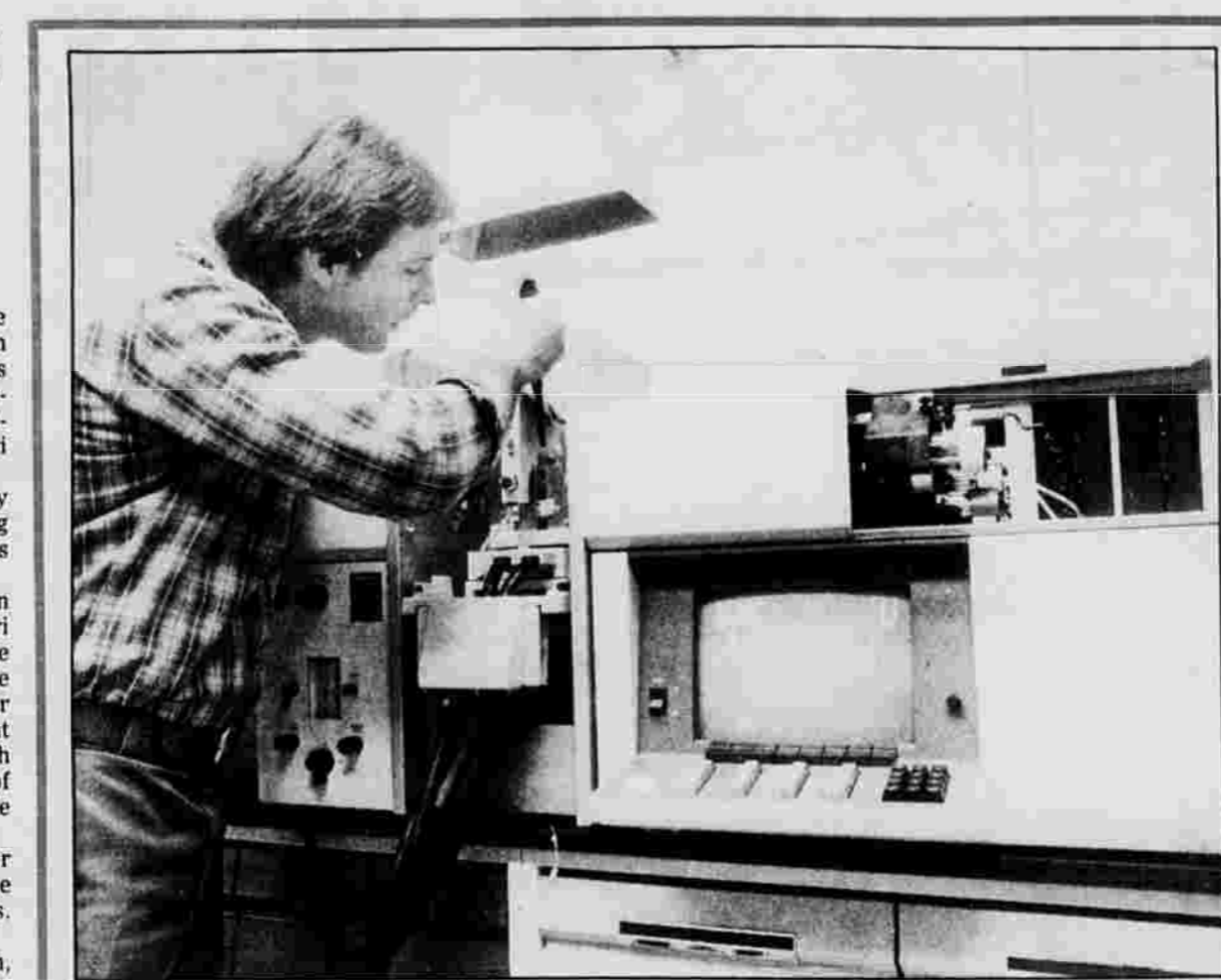
LEAD TESTING — Michael Todd, a chemist at the town's water treatment plant off Spring Street, tests water for lead content in a machine called the Parkin-Elmer 3030 Atomic Absorption Spectrophotometer. The federal Environmental Protection Agency is considering new standards for lead.
